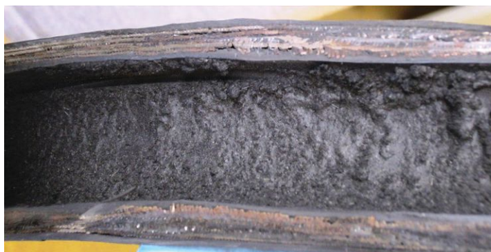
Cavitation wear and microdieseling damage. (Photos courtesy of Hegelsen Industries in Hartford, Wis., and Milwaukee School of Engineering.)
